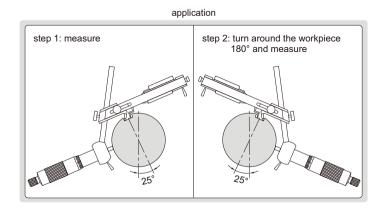
Used to measure the symmetry of shaft keyways
